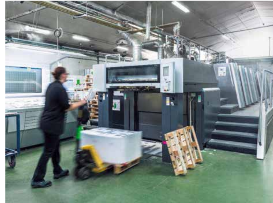
The pressroom has two almost identical 8-colour perfectors with the same format, configuration and inks to optimise production and maintenance while limiting the varieties of consumables and paper sizes. Source Cloître
