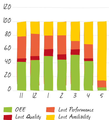
An OEE score of 70% is very good, as it shows over 90% in each measure. The average for manufacturing industries is around 60%.
