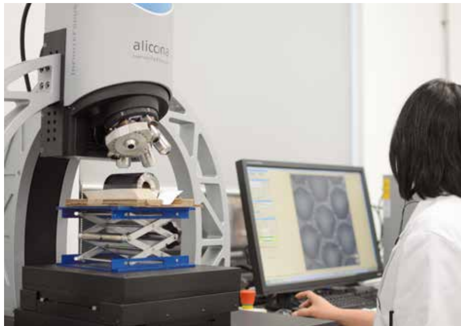
Analysing an anilox cylinder using an Alicona precision optical 3-D profiler. Source WCPC
