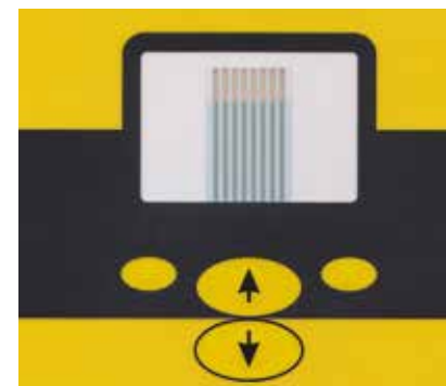
Example of a control panel combining a graphic layer, a tactile screen, 'clicky buttons' and an electric track layer. Source Screentec
