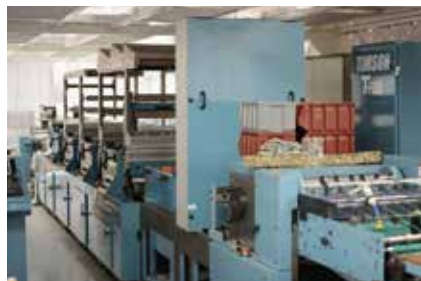
Web press for R&D, with 4 units, enhanced register control and image recognition developed for printing functional materials. Source WCPC
