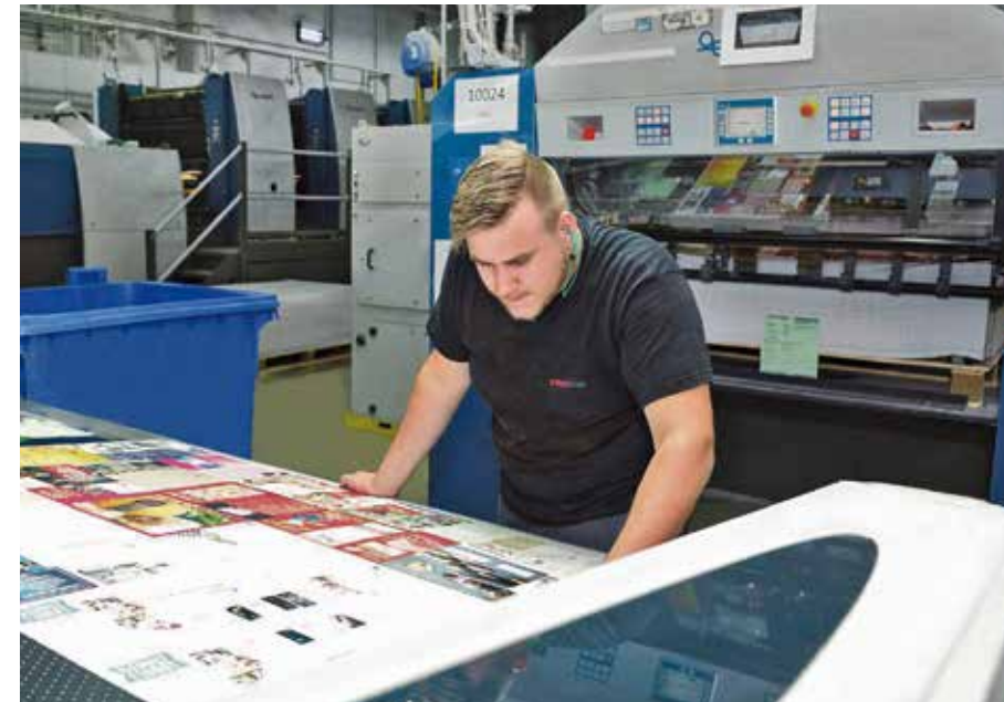
Flyeralarm prints several different jobs on the same sheet using large format presses, like this 1060 x 1450 mm Rapida 145. Source Koenig & Bauer
