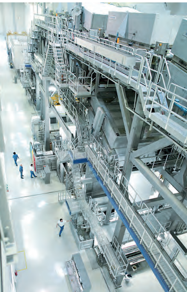
Offline Coater no.3 - Mitsubishi HiTec Paper Bielefeld Mill
